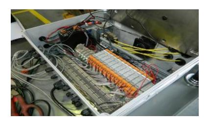
Alpha Box with C-DAQ Controller, Strain Gage Conditioners, Accelerometer Conditioners and Pressure Terminals.
